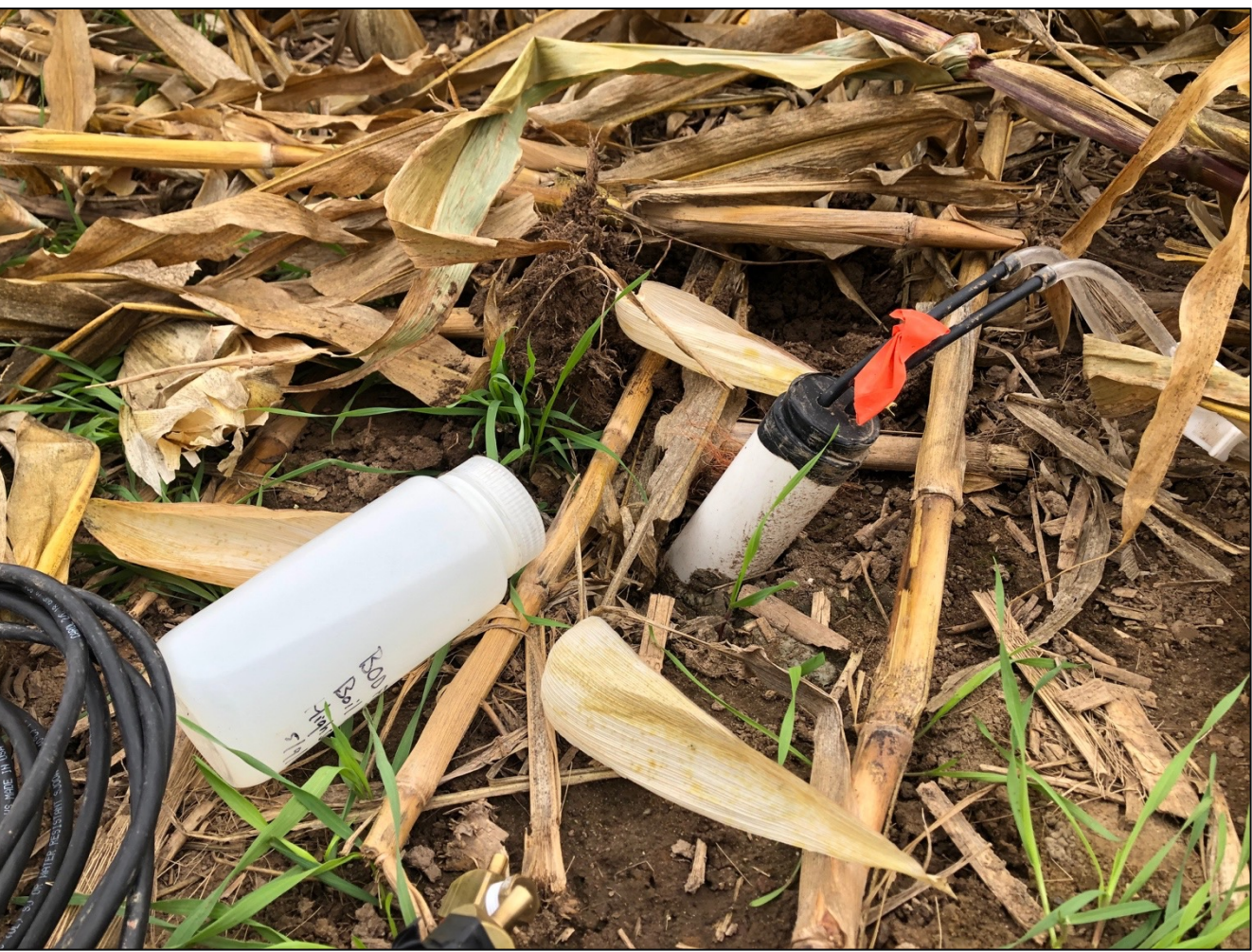
Installed suction cup lysimeter in October, 2021
