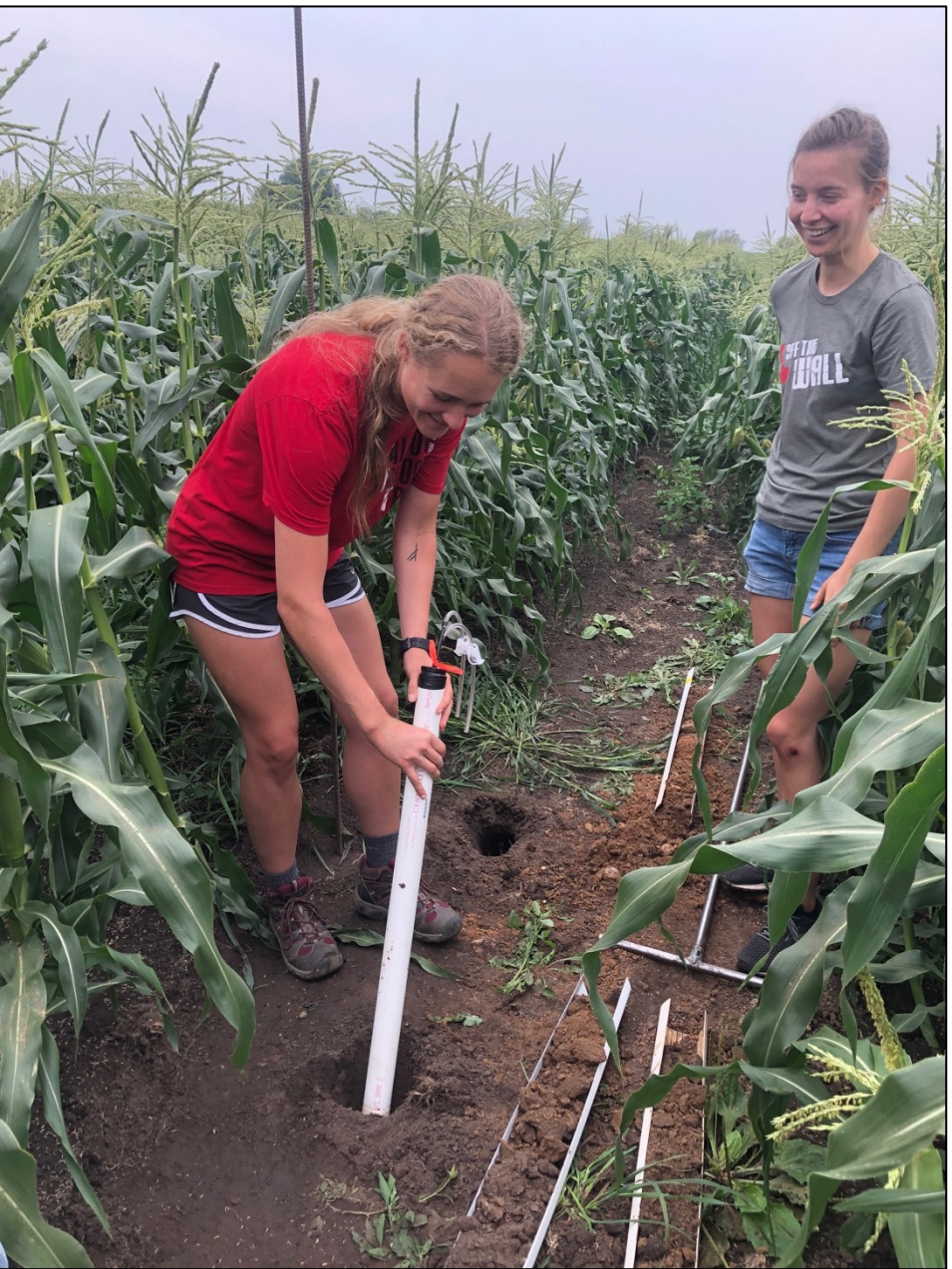
Installing suction cup lysimeters in July 2021
