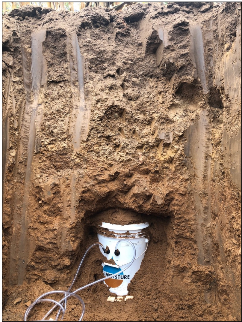
Wick lysimeter installed 4' below ground surface October, 2021
